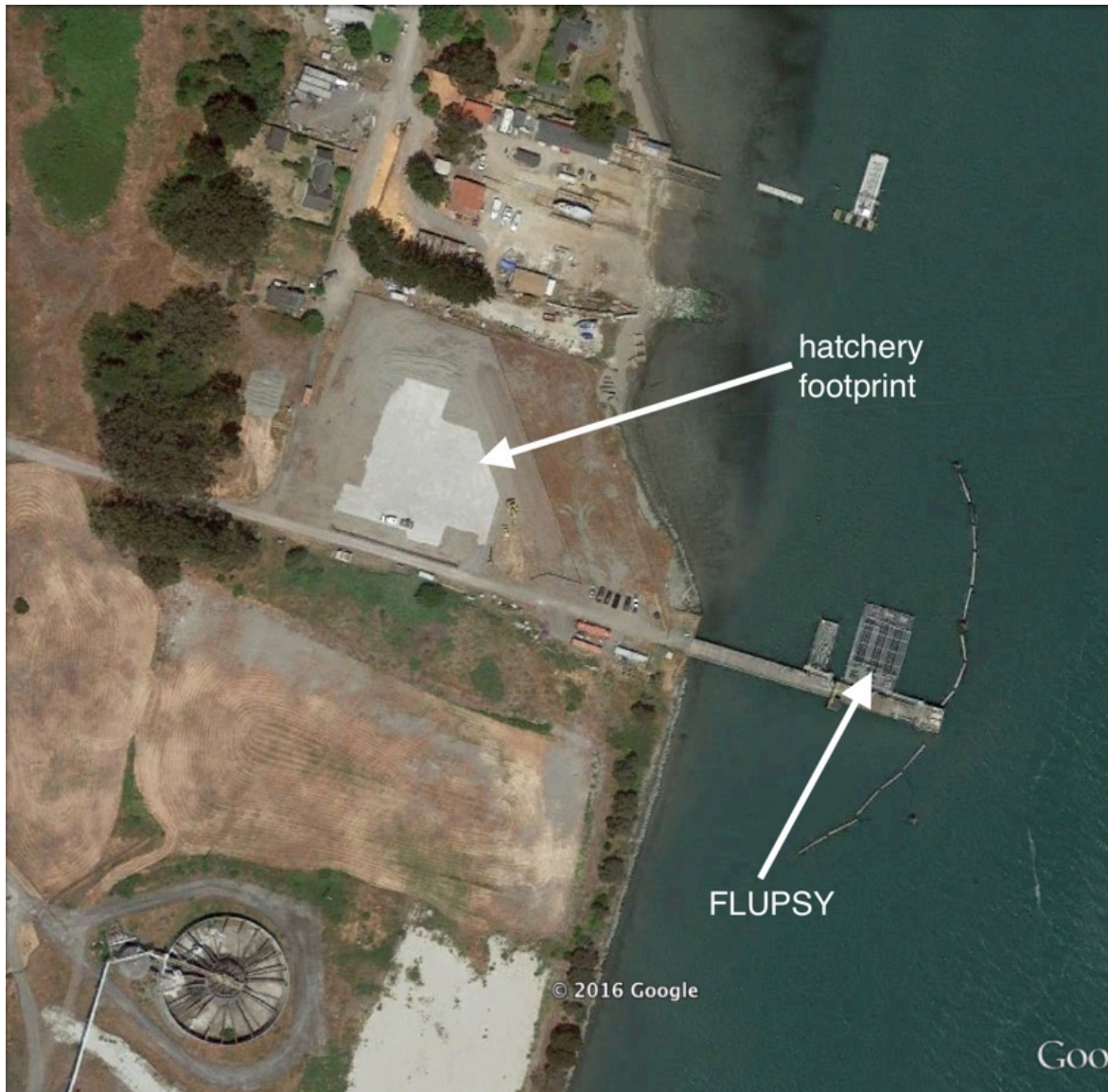
Figure 5. Google Earth view of Hog Island Oyster Company hatchery site on Humboldt Bay, showing building footprint and (FLUPSY) Floating Upwelling System where oysters are reared from spat (newly settled larvae) to the seed (juvenile) stage.
